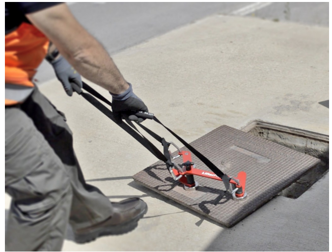
Photo 2.- LifterPro device with slings opening a lid.
